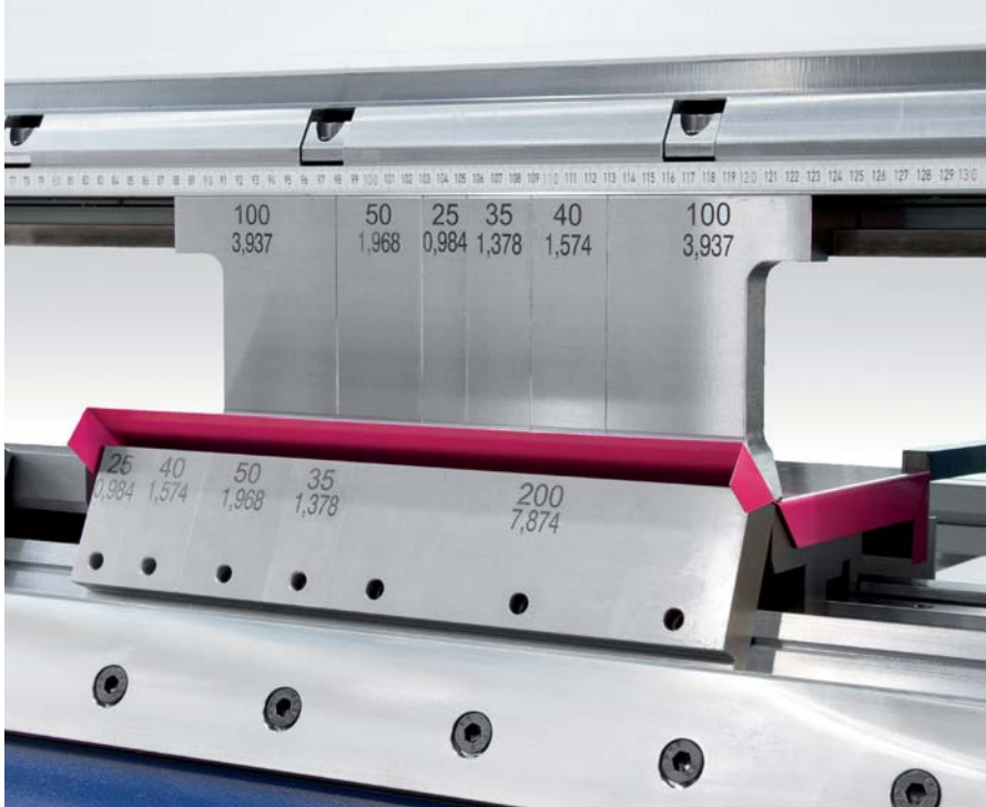
Manual clamping device: segmented tools provide flexibility for a variety of geometries
