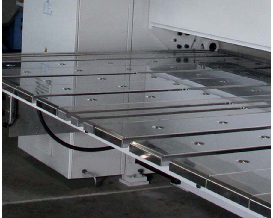
Gauge table, 1,600 mm, closed, with ball transfers
