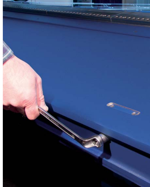
Fine tuning: crowning system manual or CNC crowning systems
