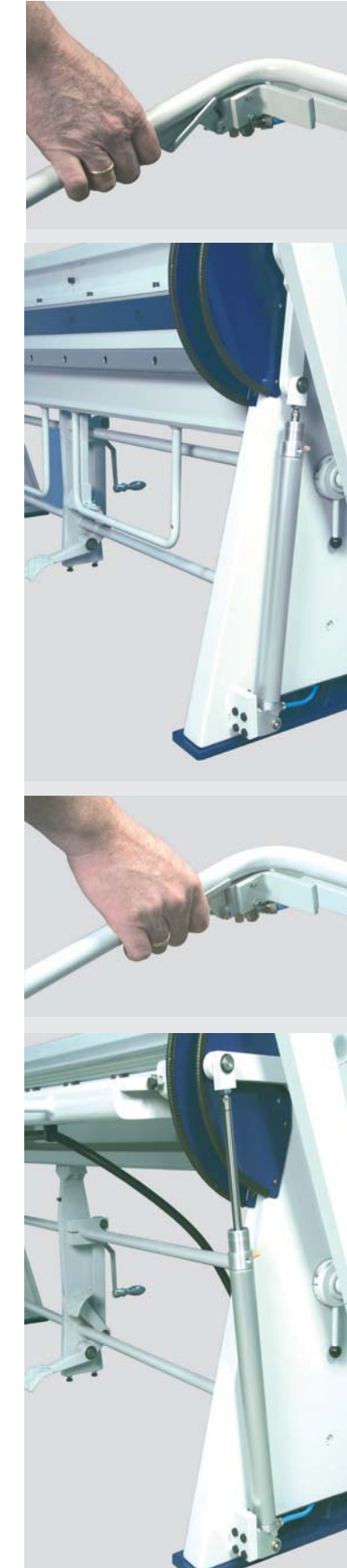
The pneumatic bending support is controlled by a finger lever on the folding beam handle. The pneumatic cylinder assists the operator in bending the piece. You only need a compressed air supply.
