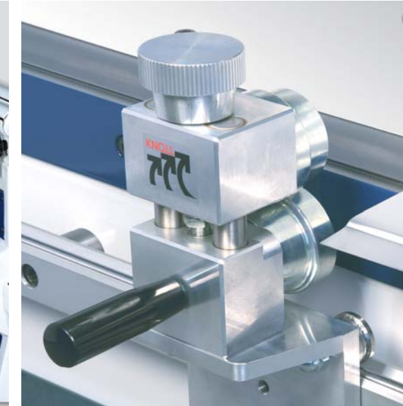
The profiling and flattening wheels are used to give the piece the required shape.
