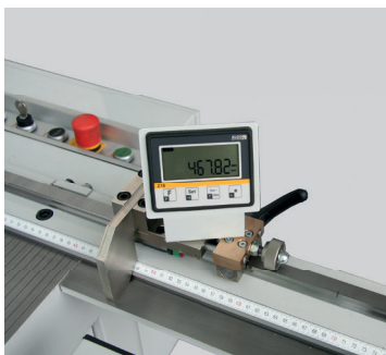
Optional: Extended angle gauge on the right with electronic length measurement system incl. lateral flip gauge on linear guide
