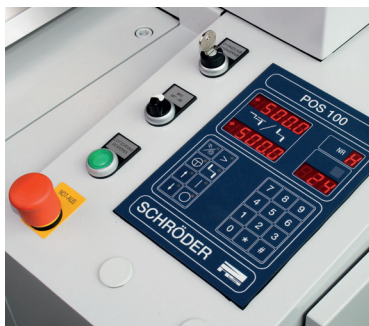
Control panel POS 100 software control
