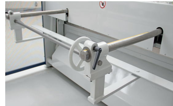
Manual back gauge, adjustment range 10 - 600 mm
