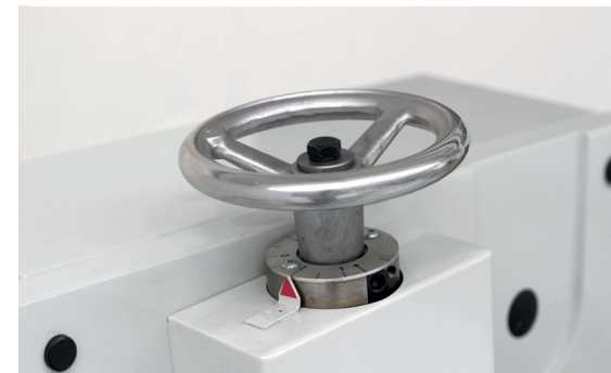
Manual blade gap adjustment
