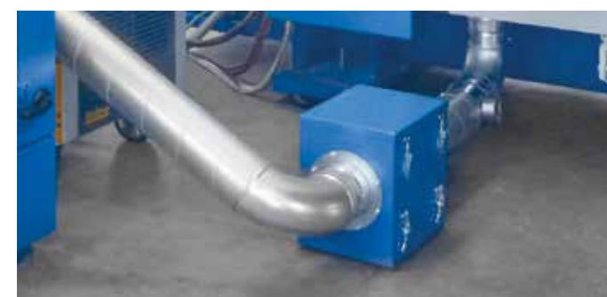
Spark separator, Temperature control and extinguishing device are standard
