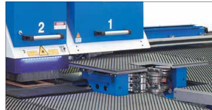
CombiLaser Multipunch with automatic tool changer
