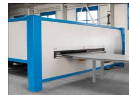
Side loading of sheets with enclosure
