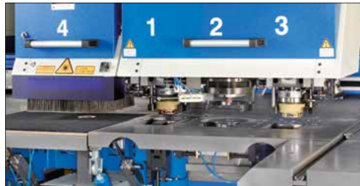
CombiLaser TRI 3-head punching machine with 2xRevotool (head 1 + 3) and rotation / index (head 2)
