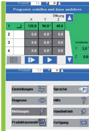
Simple icons and alphanumeric data are used to describe the bending program.
