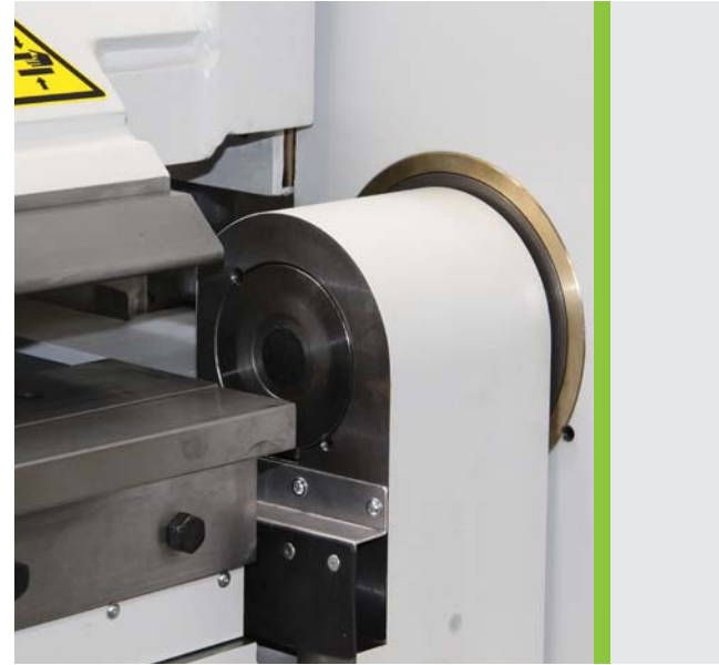
Automatic adjustment of folding beam and bending center position relative to material for accurate control over bending radius. Automated crowning completes the settings needed for accurate, repeatable forms.
